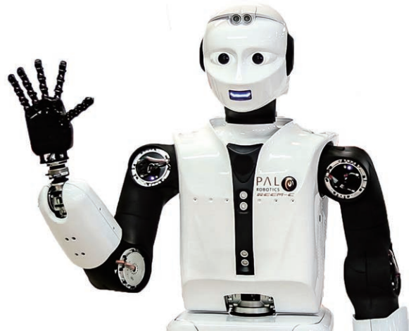
肘部关节和腕部关节安装有AksIM和Orbis磁旋转编码器的REEM-C
