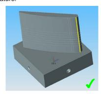
The parallel curves defining a patch should be relatively straight in the surface space.
