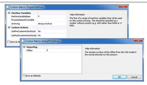
As a minimum, the *ProcessStatusNCVariable* property (in *Custom Macro: ProgramSettings*) should be set to a free NC variable. When the Freeform Surface program is run on a machine tool, this variable will be set to 0 (zero) to indicate success, or a non-zero value to indicate failure.
