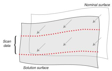
Solution surface data is saved to disk – which can subsequently be accessed for downstream processing – or sampled to access measurement data from the individual part such as:
