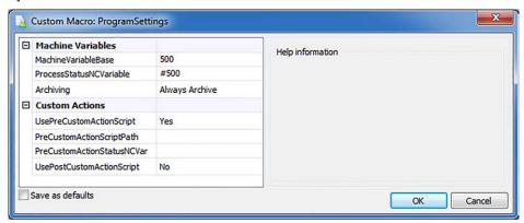
When turned on, the corresponding *CustomActionScriptPath* property should define the full path to the script or executable as seen from the external data processor. The corresponding *CustomActionStatusNCVar* properties should be configured to define free NC variables.
