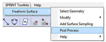
Settings in the *Freeform Surface Post Process* dialog box must be configured, ensuring that the specified *Machine Definition File (.RenMF)* matches the .RenMF file used on the CNC machine tool.
