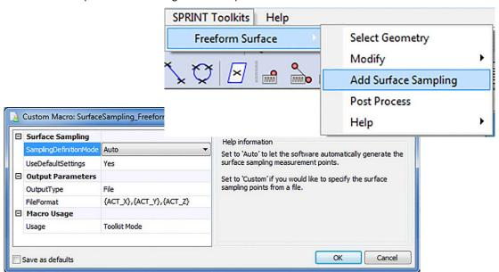
The points at which the solution surface should be sampled can be automatically generated by the Toolkit or specified by the user (via a comma-separated file containing three columns corresponding to the XYZ positions of the sampling points on the nominal surface).
