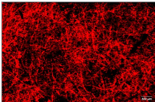
Figure 5a. Image of microcrystalline cellulose distributed, with a fibrous structure, within the patch matrix
