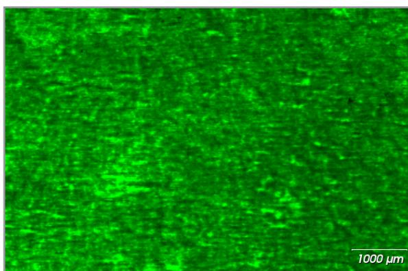
Figure 5c. Image of nicotine and the EVA-based matrix material, distributed together. Variations in the intensity of green correlate to differences in the uniformity of these materials
