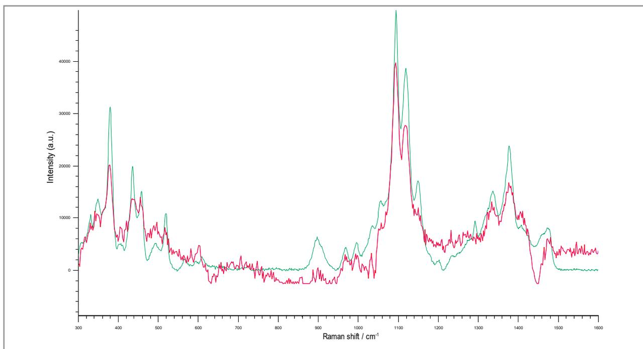
Figure 4. Identifying formulation components using Spectrum Search in Renishaw's WiRE software - an Empty Modelling component spectrum (red), resolved from the map measurement of the nicotine patch, matches to a library spectrum of microcrystalline cellulose (green)
