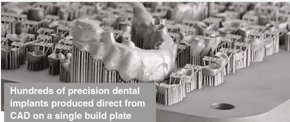
Hundreds of precision dental implants produced direct from CAD on a single build plate
