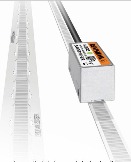
Incorporating industry-proven technology from the RESOLUTE™ encoder series, EVOLUTE™ is a true-absolute 50 µm scale period optical encoder with wide installation tolerances and high immunity to dirt.
