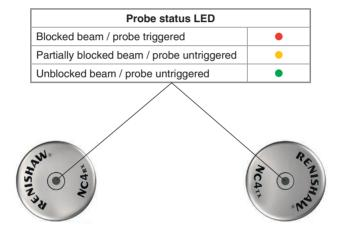
For more information on these LED sequences and modes of operation, see the *NC4 separate* non-contact tool setting system installation and maintenance guide (Renishaw part no. H-4114-8500).
