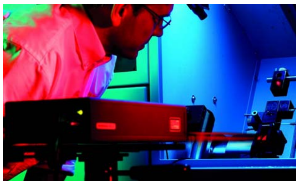
Fig 11 – calibrating a turning centre with a laser interferometer
