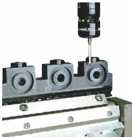
Fig 7 – measuring a calibrated 'artefact', which removes thermal and geometry errors from on-machine inspection
