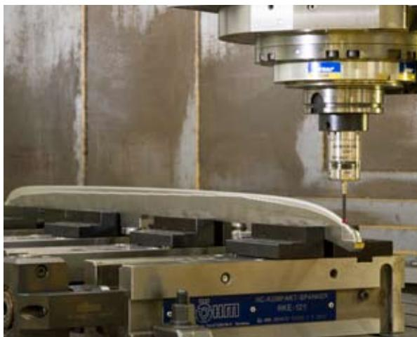
Once the data had been captured, both DXF and IGES files were created and sent electronically to Sescoi, who created a CAD/CAM program for a Siemens Sinumerik machine tool controller fitted to a DMG CNC milling machine located at tooling manufacturer Iscar. Following machining, the finished blades were checked for form using the Renishaw OMP400 touch probe, a strain gauge based product which allows highly accurate on-machine measurement to be performed.
