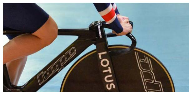
British Cycling with Renishaw 3D printed titanium and aluminium handlebar (image courtesy of SWPix)
