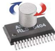
Figure 1: OnAxis™ encoder, consisting of a magnet and a chip containing sensors and evaluating electronics.
