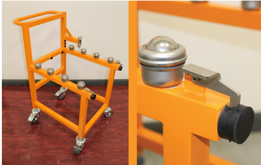
Figure 24 Hopper trolley and latch
