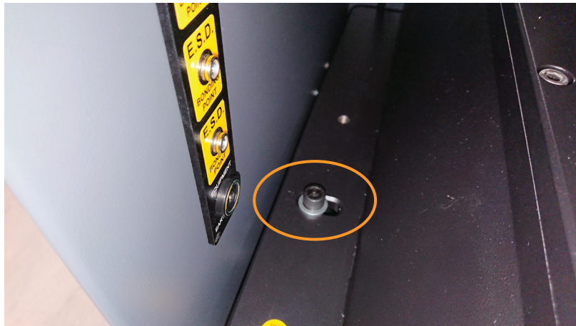
Figure 28 Bolt securing the hopper to the AM system
