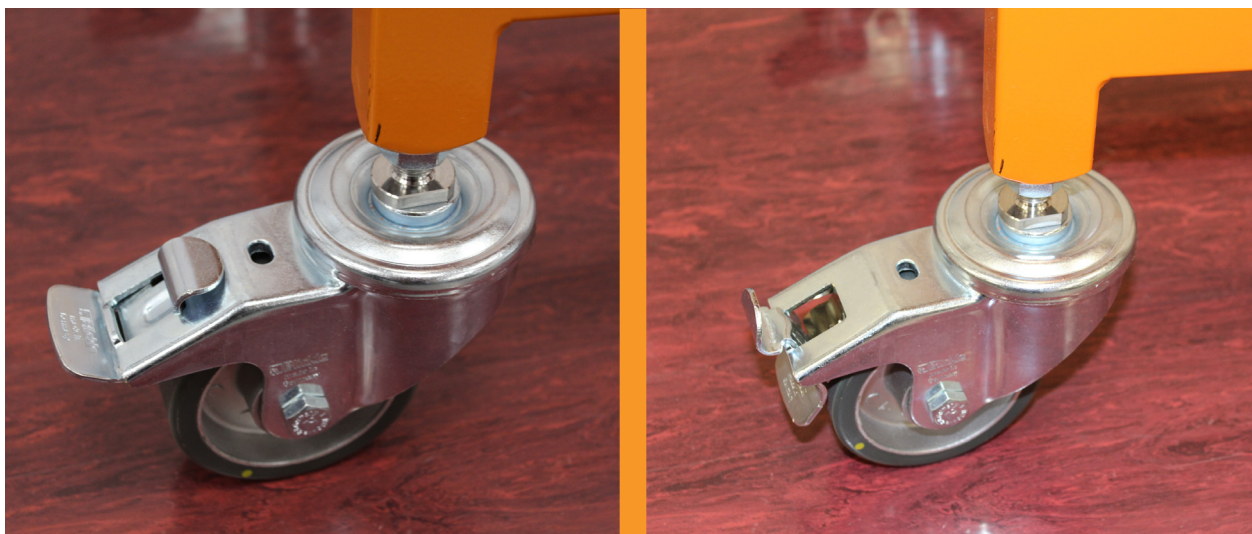
Figure 26 Hopper trolley braked castors – unlocked (left) and locked (right)
