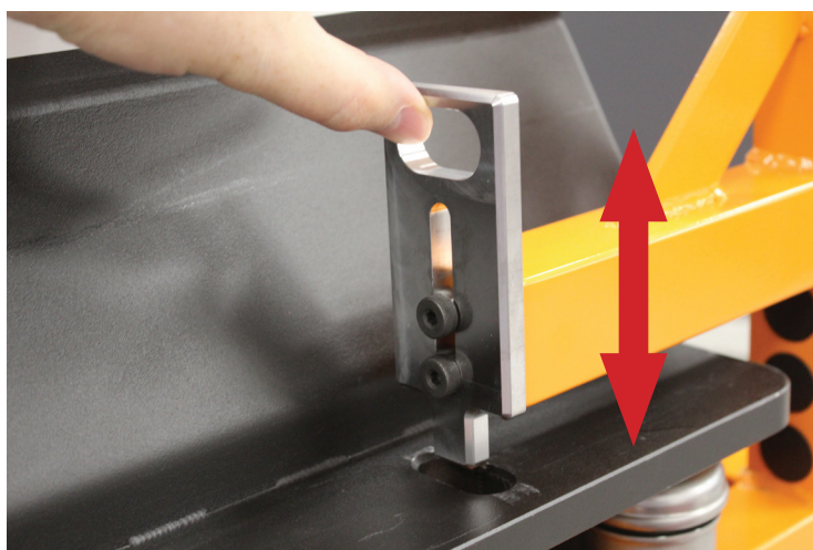
Figure 14 Hopper to hopper trolley latch – raised
