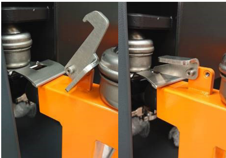
Figure 25 Hopper trolley to AM system latch, raised (left) and engaged with receiving bracket (right)
