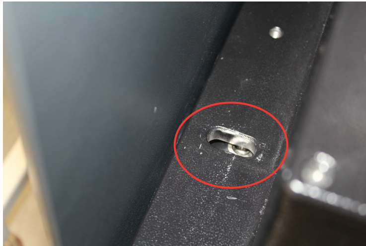
Figure 15 Slot machined into hopper left-hand side
