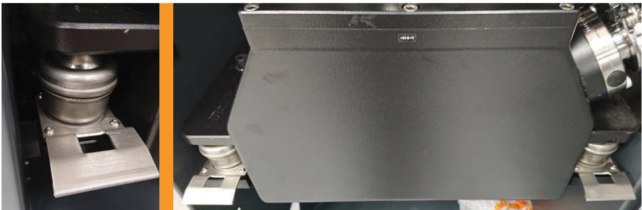
Figure 23 Transfer roller and securing fasteners (left) and left and right transfer rollers (right)
