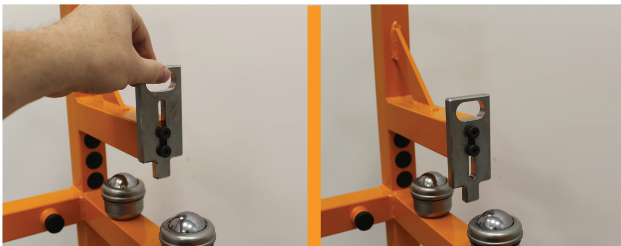
Figure 32 Hopper to hopper trolley retaining latch and raised
