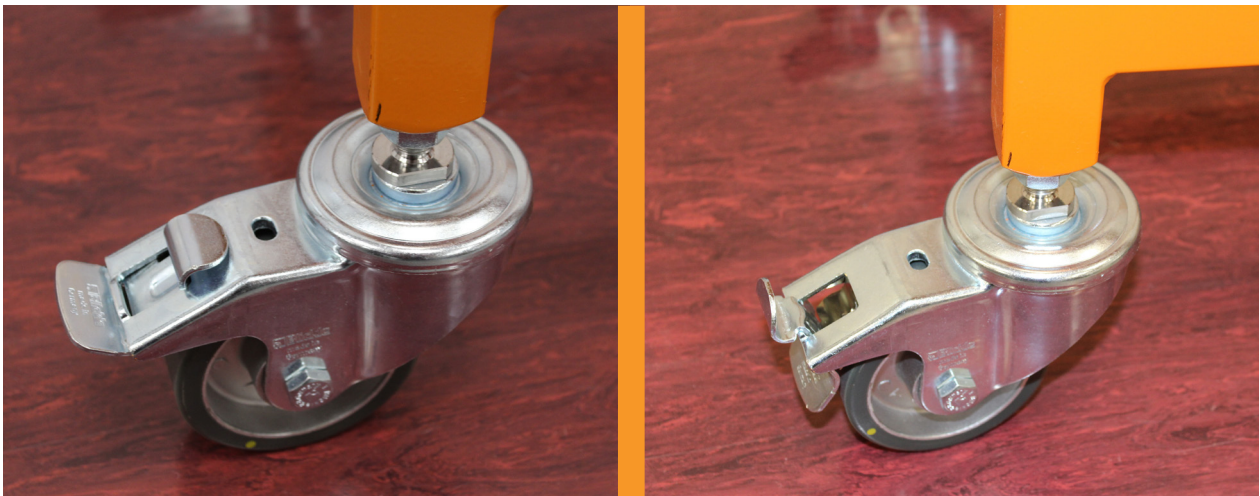
Figure 34 Hopper trolley braked castors – unlocked (left) and locked (right)
