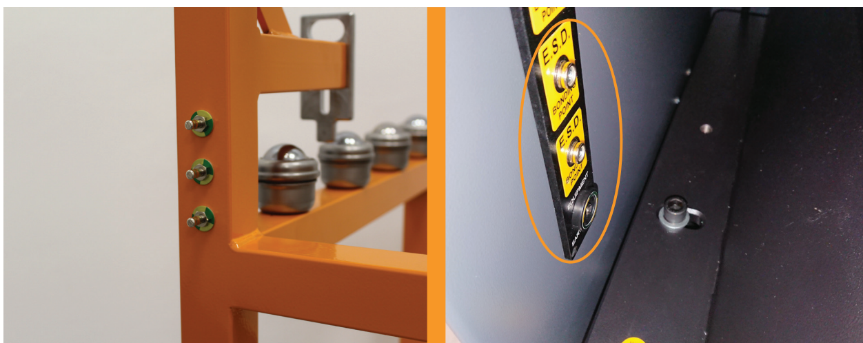
Figure 27 Hopper trolley ESD connection points (left) and AM system ESD connection points (right)
