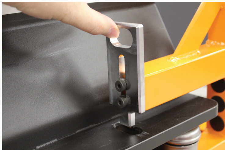
Figure 29 Hopper to hopper trolley retaining latch – raised
