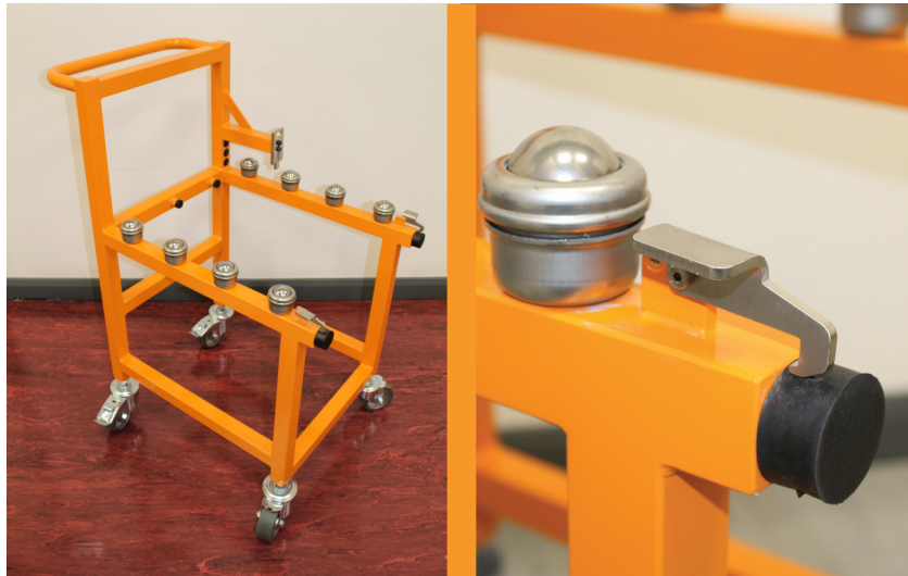
Figure 20 Hopper trolley and latch
