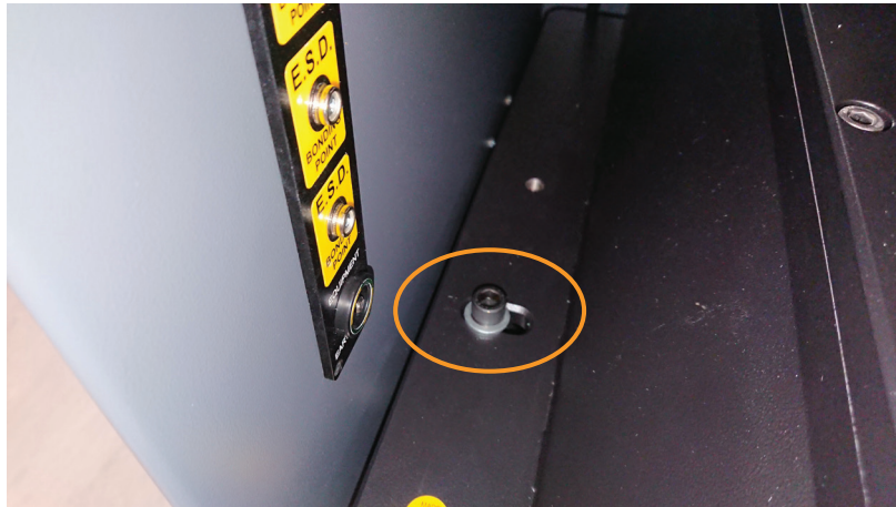
Figure 22 Bolt securing the hopper to the AM system
