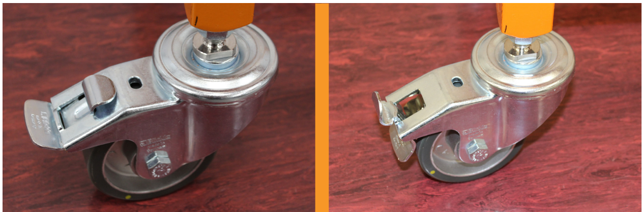
Figure 12 Hopper trolley rear locking castor – unlocked (left) and locked (right)
