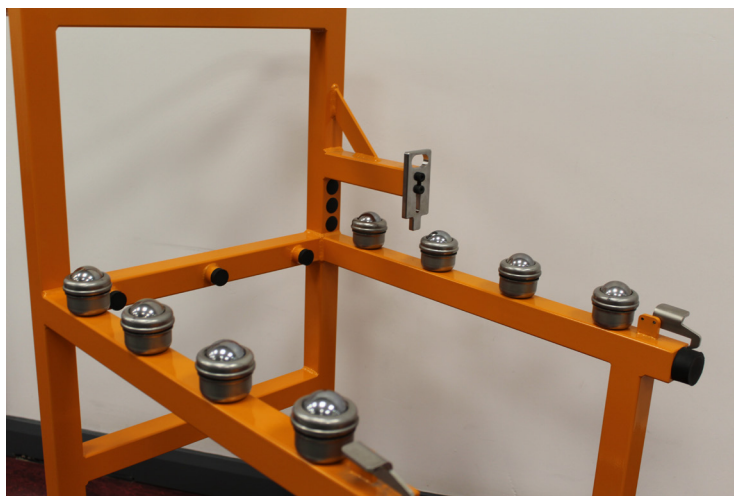
Figure 17 Eight rollers to ease loading
