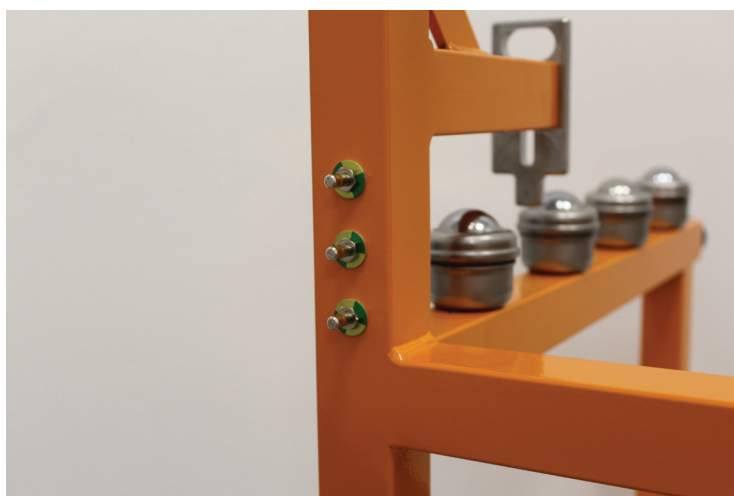
Figure 36 ESD cable connection point
