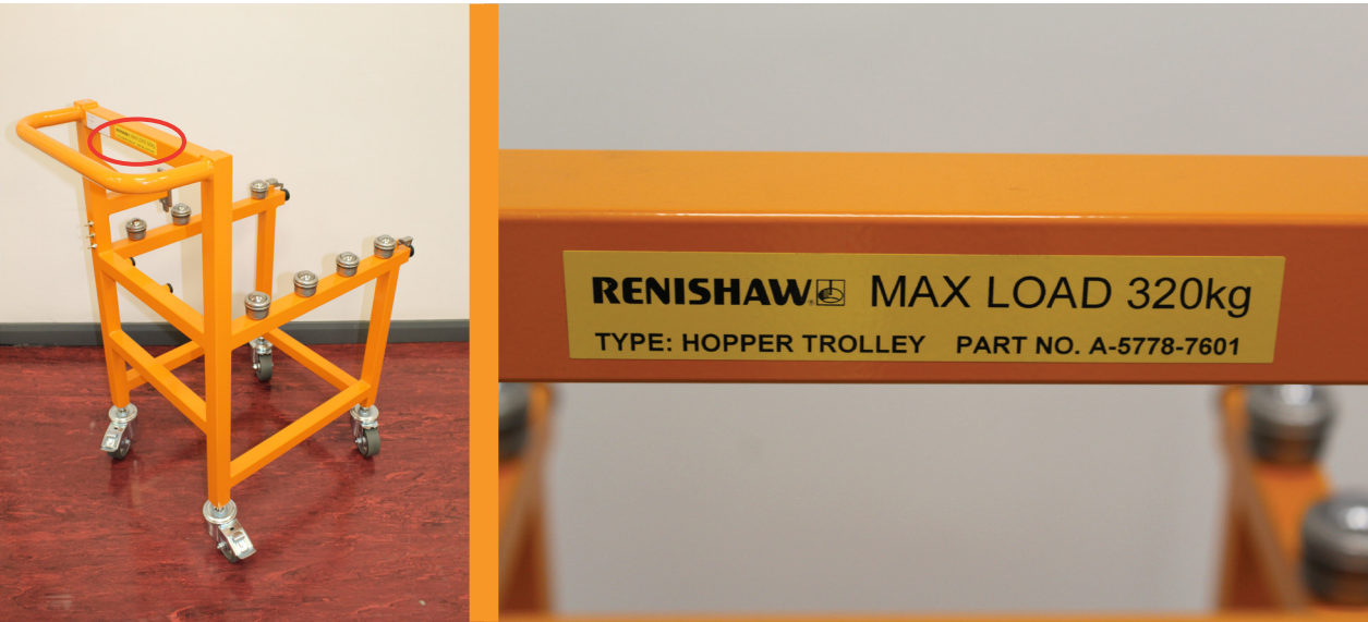
Figure 4 Renishaw hopper trolley specification and capacity plate and location
