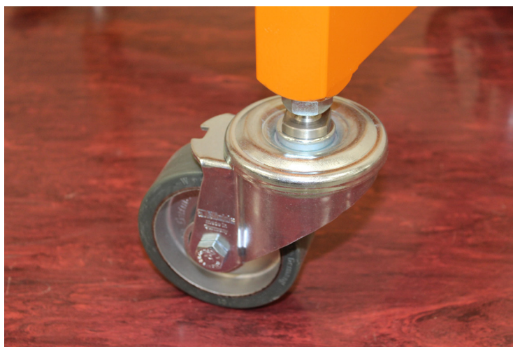
Figure 35 Hopper trolley front castor
