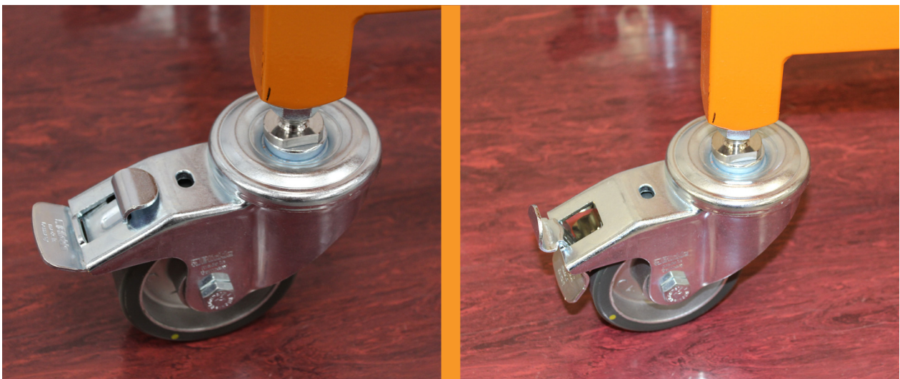
Figure 21 Hopper trolley braked castors – unlocked (left) and locked (right)
