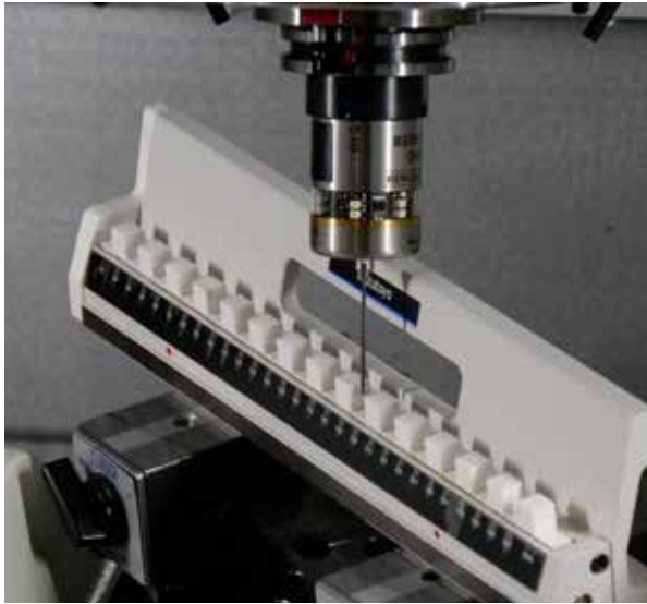
KES is also an advocate of Renishaw's machine tool probing systems
