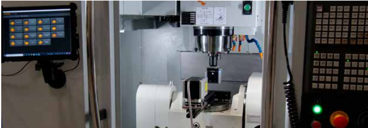
KES uses the XM-60 on both its CNC machine tools and CMMs to perform volumetric compensation
