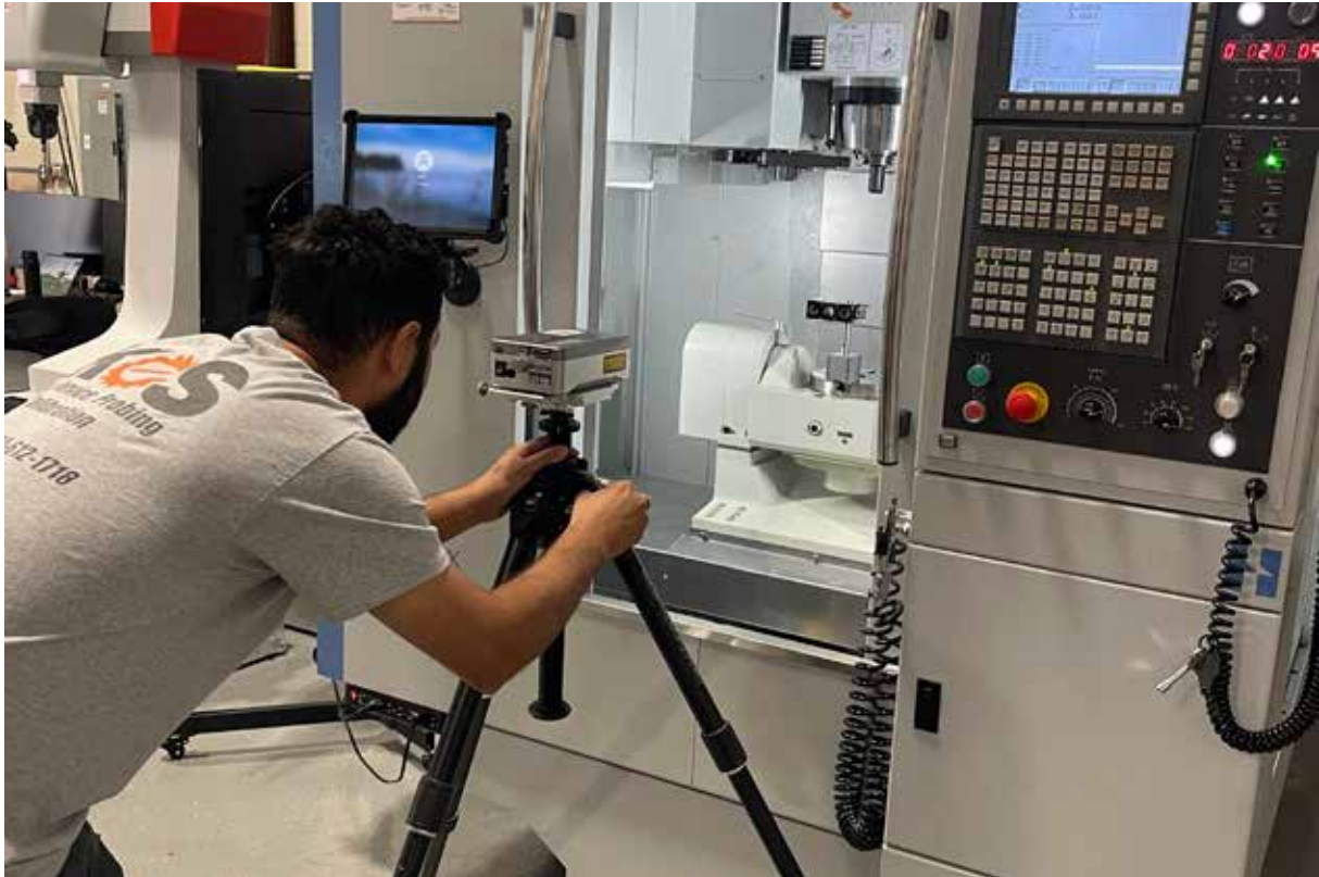
Renishaw's XL-80 laser system on a CNC machine tool
