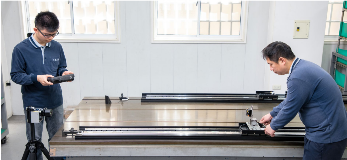
Validation of precision linear stages with the XK10 alignment laser system
