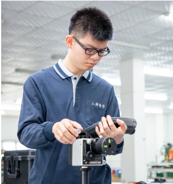
Smooth Precision engineer using a wireless display unit to align the XK10
