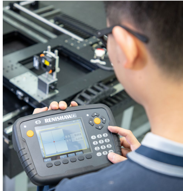
XK10 display unit records measurements and displays instant readings so users can make adjustments on the fly
