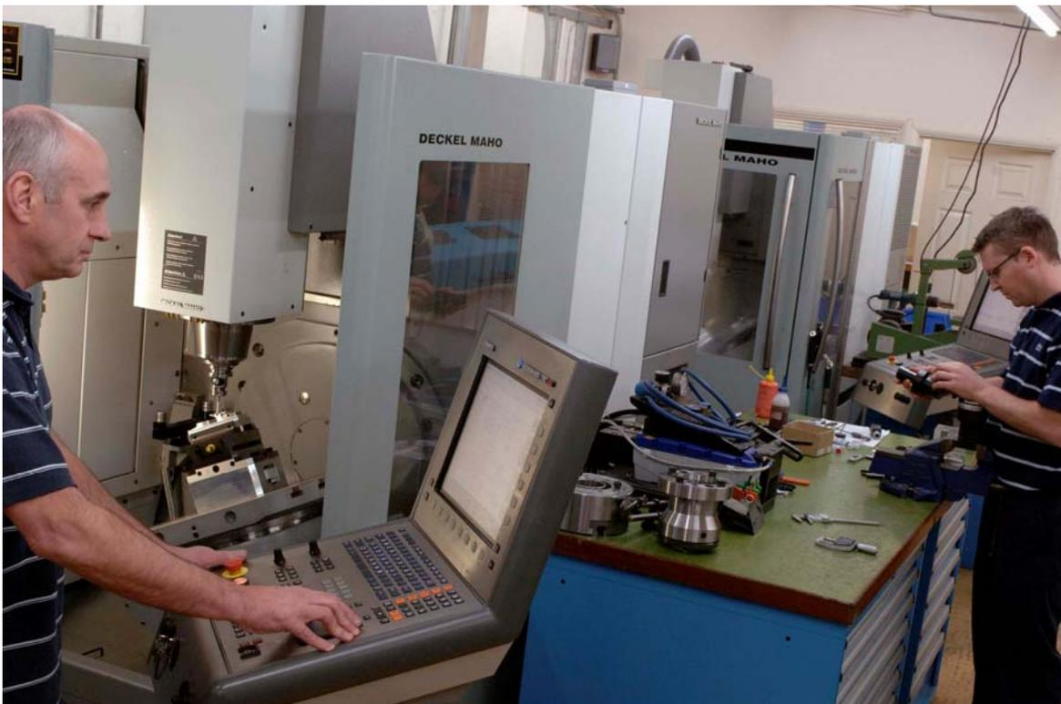
Jobs are loaded onto the DMG DMU-50 machines on small pallets and require multiple tool changes
