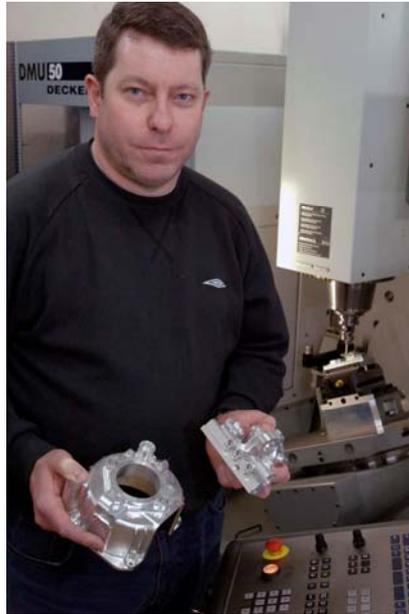
John Kenny, with specialised parts produced on DMG DMU-50 VMCs
