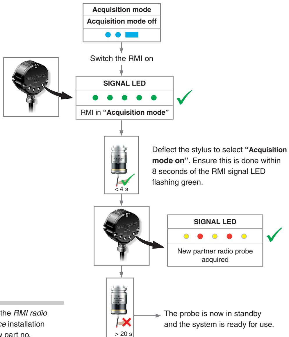
**NOTE:** Refer to the *RMI radio machine interface* installation guide (Renishaw part no. H-4113-8554) when partnering the RMP600.
