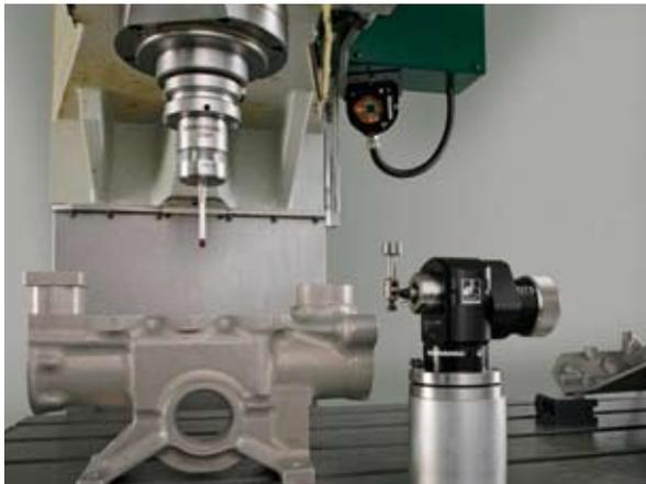
A typical twin probe system will comprise the new Renishaw OTS tool setter and Renishaw OMP40-2 inspection probe, but other compatible spindle-mounted touch probes with modulated optical transmission may also be used. The cableless tool setter design is particularly suitable for machines with twin pallets or rotary tables, which historically have proven challenging for installations of hard-wired tool setters.
