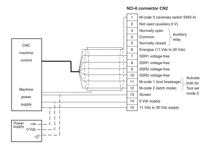
**CAUTION:** If using SSR2 as an oscillating or pulsed output for a trigger signal to the control, the level output SSR1 must be used to guarantee a reliable probe status check.
