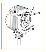
CAUTION: DO NOT remove the window by twisting or rotating.
