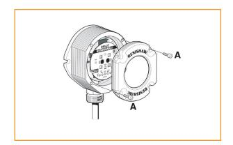
Tighten each screw a few turns at a time to pull the window up evenly. When it is clear of the body, remove the window and screws completely.
