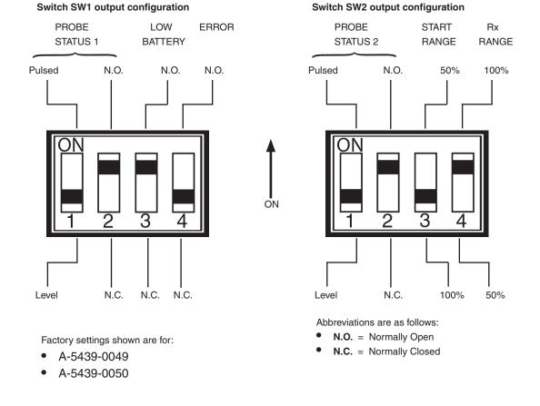
**CAUTION:** Exercise caution when using error or probe SSR in N.O. mode as a wiring fault could cause a loss of error condition and therefore could result in a non-fail safe condition.
