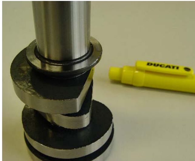
The Desmodromic camshaft is not conventional, and has been designed with special 'lifting ramps'
