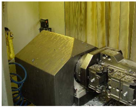
Renishaw non-contact laser system mounted outside the working envelope of the machine
