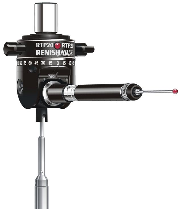
RTP20 integral TP20 probe mount optimises the working volume of the CMM and provides compatibility with all existing TP20 modules. Although modules can be changed manually, the RTP20 can be used with the MCR20 module change rack, allowing fully automated module changing.
