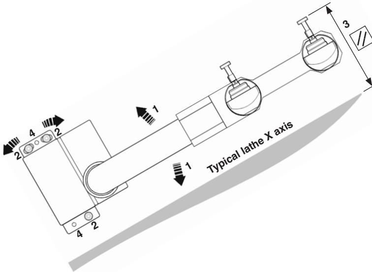
1. Rotate arm on bottom mounting screw to set stylus alignment.
