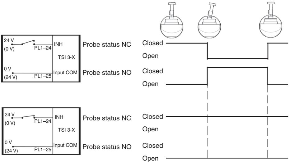
**NOTE:** The probe status LED will still function when inhibit is active.
