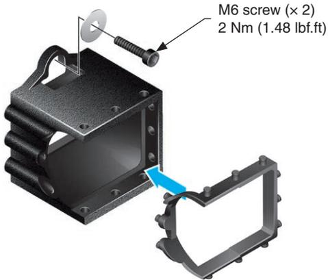
1. Fit the probe pocket(s) using the probe pocket fixing kit supplied (M6 screws and washers). Ensure the screws are loose (finger-tight).
