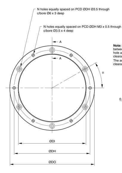
Note:  $\theta$  is the angle between one tapped hole and the adjacent clearance hole. The angle between two clearance holes is  $2\theta$ .
