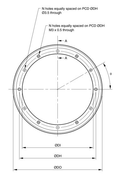
Note:  $\theta$  is the angle between one tapped hole and the adjacent clearance hole.
