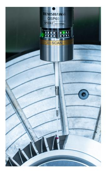
Information in this document is based on an existing installation of a Renishaw OSP60 probe with SPRINT technology.
