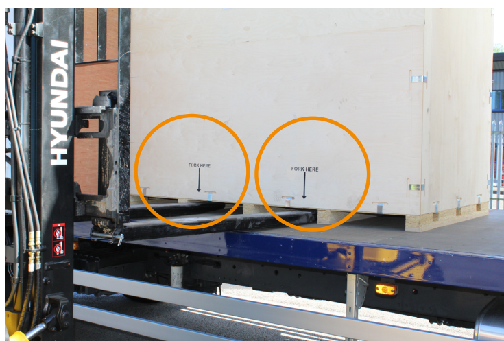
Figure 43 Lifting points on the crate
