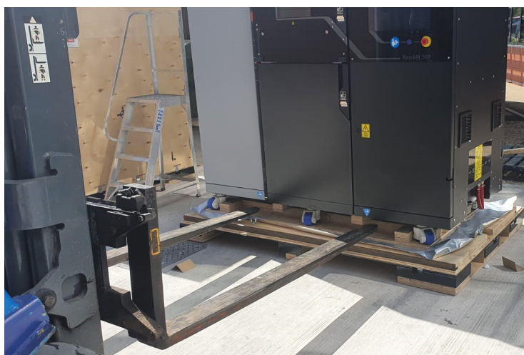
Figure 62 Align forks with forklift lifting point symbols
