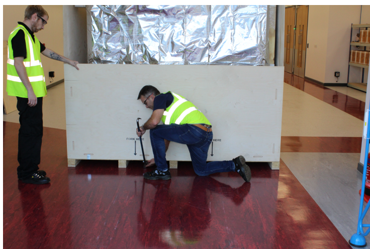
Figure 49 Supporting and removing front lower panel clips
