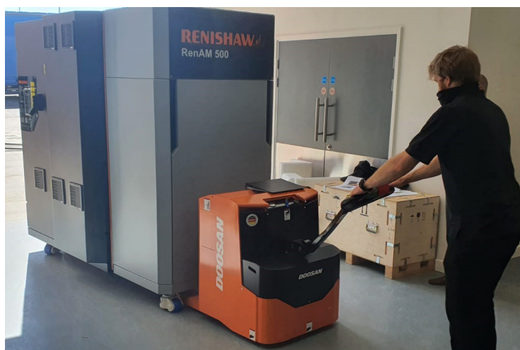
Figure 65 Moving the system using a powered pallet truck
