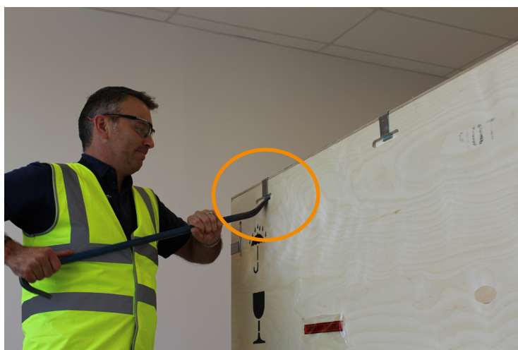
Figure 45 Removing the clips that secure the lid
