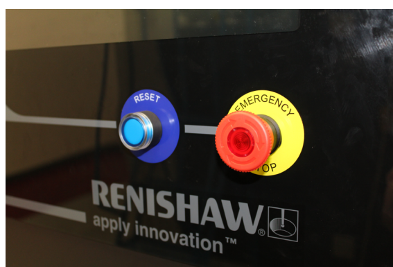
Figure 4 “Emergency Stop” button on front of RenAM 500 series system
