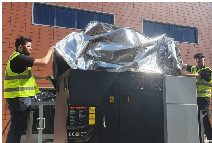
Figure 59 Removing the foil bag fitted over the system
