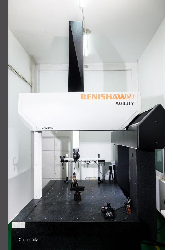
Renishaw's AGILITY® CMM was suggested as an ideal solution for DMNC-EDM. Not only is it designed to deliver all the advantages of the REVO system's range of specialised sensors, but also because its unique 5-axis measurement technology and synchronised motion control deliver ultra-high measurement speed and increase inspection throughput.
