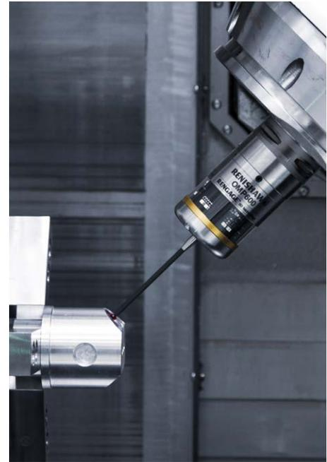
图14: OMP600应变片式工件测头
