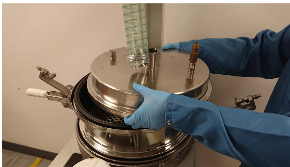
Figura 25 Remova a tampa
