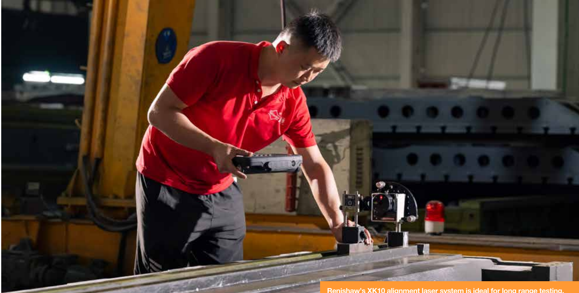
Renishaw's XK10 alignment laser system is ideal for long range testing.
