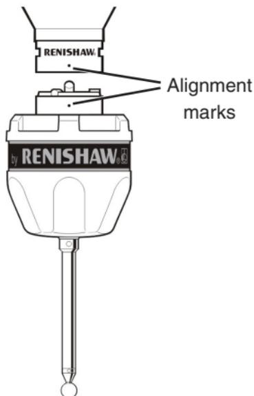
**Figure 5 - NDI AUTOsense module alignment**
