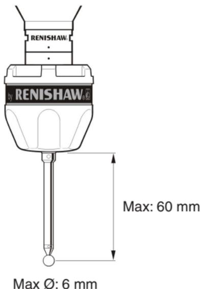
**Figure 7** - Recommended stylus limits
