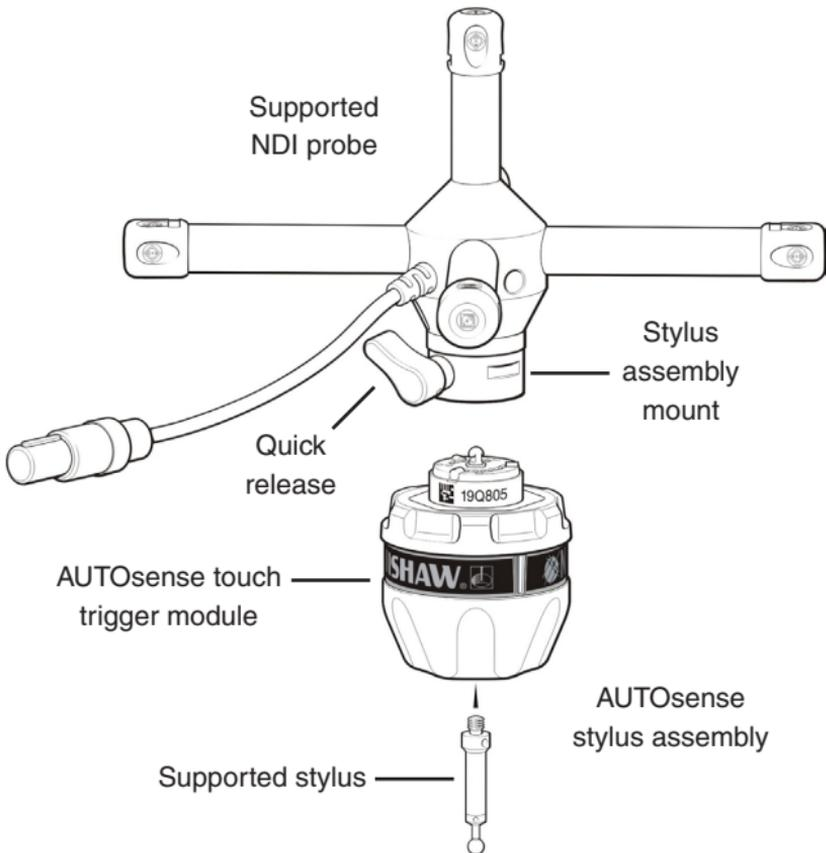
**Figure 3 - The NDI AUTOsense system components**
