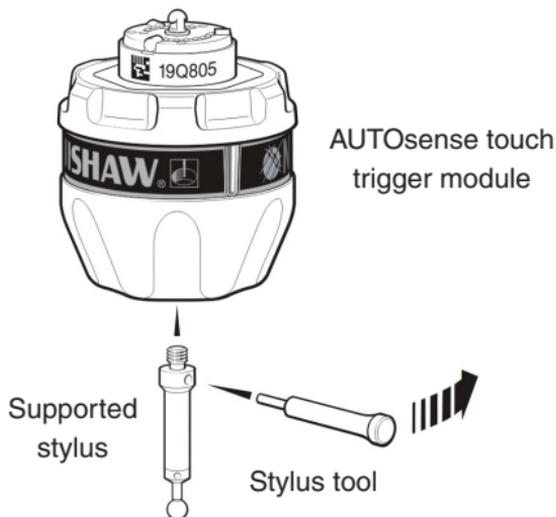
**Figure 4 - Stylus fitting**
