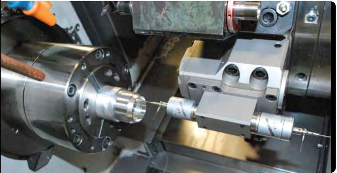
The success the company achieved using on-machine probing on its VMCs spurred it to apply probing to turn-mills such as this one.
