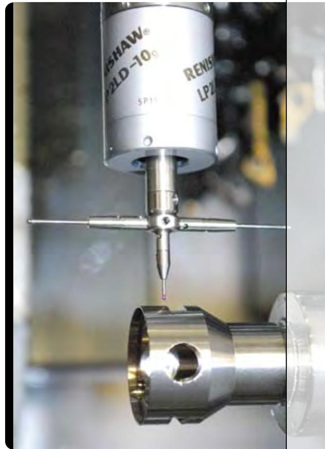
This probe installs on the platen of a Swiss-type lathe so both X- and Y-axis movement is possible. That motion combined with the probe's three styli allows access to features of parts located on both the main and secondary spindles.
