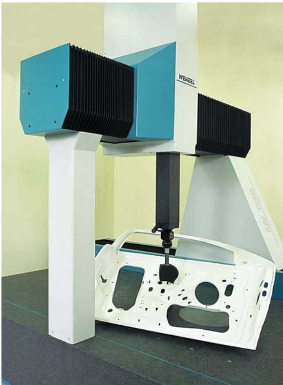
2 – Part digitising on a Travelling Bridge CMM equipped with an Optical Sensor fitted on an indexable wrist
