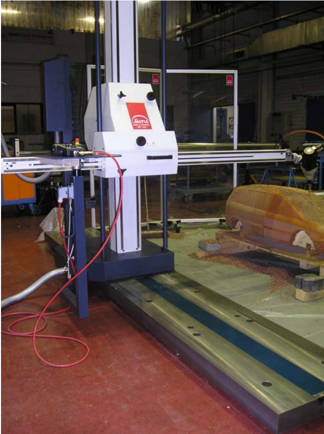
4 – Light Milling of a part by means of an Horizontal Arm CMM
