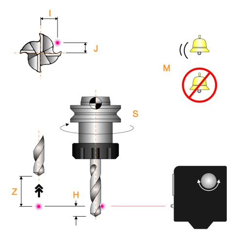
Typically, a tool needs to be checked after a machining operation, to verify that it is not broken, before the next tool is selected.
