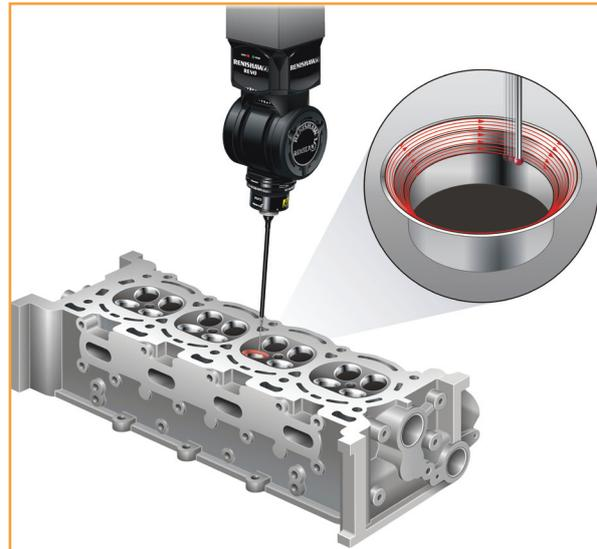
REVO® valve seat and stem scanning on generic head
