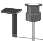
it comes into contact with a tool. Failure to contact the tool therefore leads to the conclusion that it is broken.
