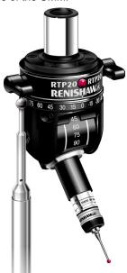
The existing range of TP20 modules provides a selection of trigger forces and directional sensing options as well as increased reach with EM1 and EM2 extension bars. The magnetic kinematic joint provides crash protection in the event of accidental collision.
