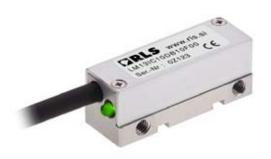
Engineered for extreme service, LM13 encoders handle operating temperatures from 10 °C to 80 °C, providing waterproof sealing to IP68 and high resistance to shock, vibration and pressure. Frictionless operation eliminates wear, while reducing system inertia and hysteresis for high precision at high speeds and accelerations.
