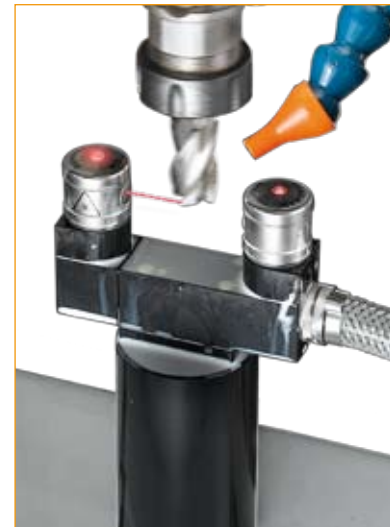
NC4 compact checking a tool for breakage
