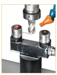
NC4 compact checking a tool for breakage
