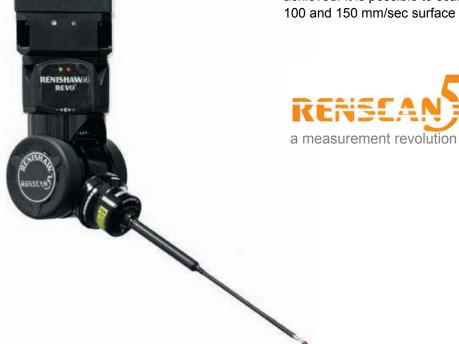
When a five axis measuring system is used, much of the unwanted CMM dynamic error is removed because the measuring head performs most of the work. As the head is much lighter and more dynamic than the CMM, with a significantly better frequency response, it is able to quickly follow changes in the part geometry without introducing harmful dynamic errors. This allows the CMM to do what it is best designed to do – move at constant velocity in a single vector while measuring.
