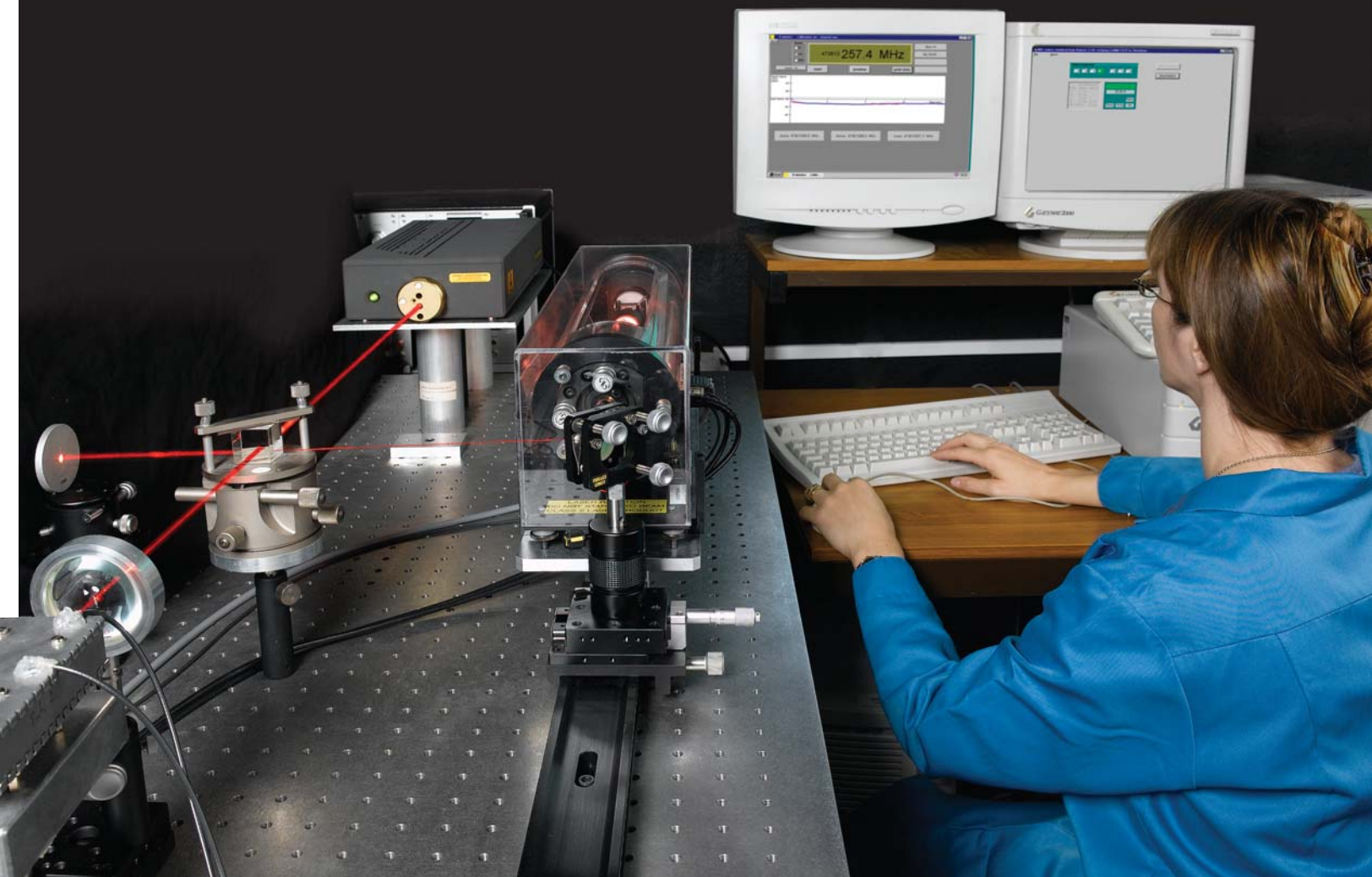
Calibrating Renishaw's ML10 Gold Standard laser systems against an iodine stabilised reference laser which is regularly calibrated at the National Physical Laboratory (NPL), UK
