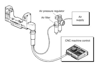
NCi-4 connected to a typical non-contact tool setting probe
