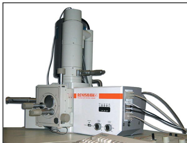
Figure 3 High vacuum version of the structural and chemical analyser interface coupled to a JEOL SEM
