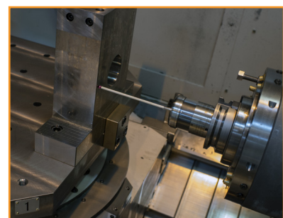
Renishaw's RMP60 touch-trigger probe can be used for component setting or inspection on machining centres.
