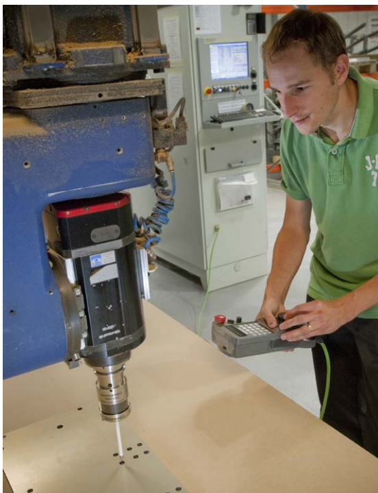
The 5-axis CMS router fitted with a RMP600 touch probe is used to machine AW159 components and other tooling in-house
