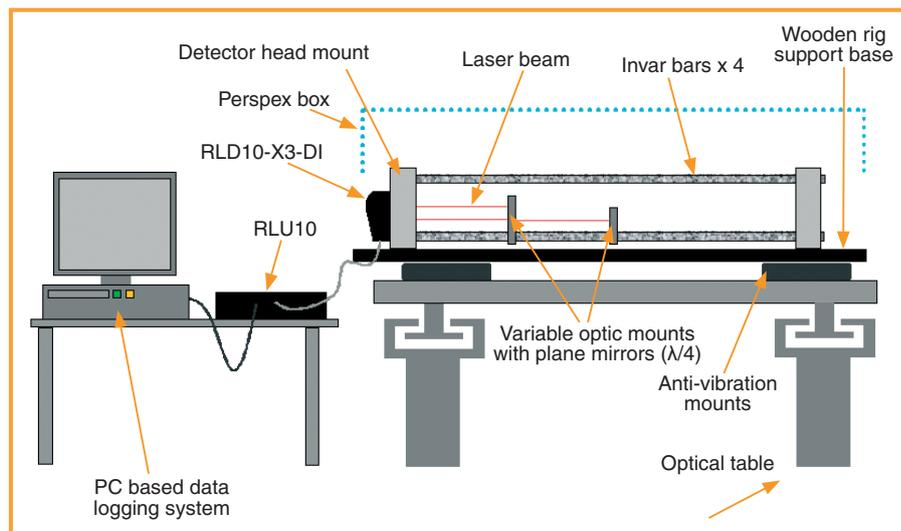
Figure 4: test rig set-up
