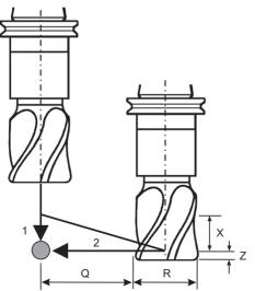
The effective radius/diameter is written into the tool offset register. If the controller has separate wear and geometry registers, the wear register is zeroed and the radius/diameter value is placed in the geometry register.
