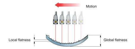
Flatness is usually specified as a 'peak to valley' figure quoted as a fraction of a wavelength over a particular length. For example:
