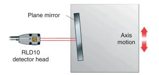
Orthogonality error, caused when perpendicular mirror axes are not truly orthogonal to each other
