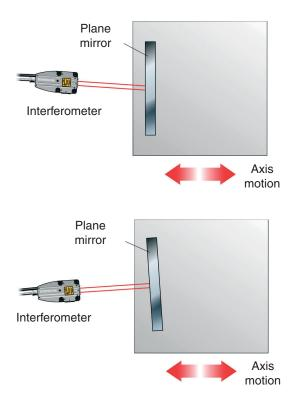
Cosine error = axis of motion length (1 - cosine  $\Phi$ )
