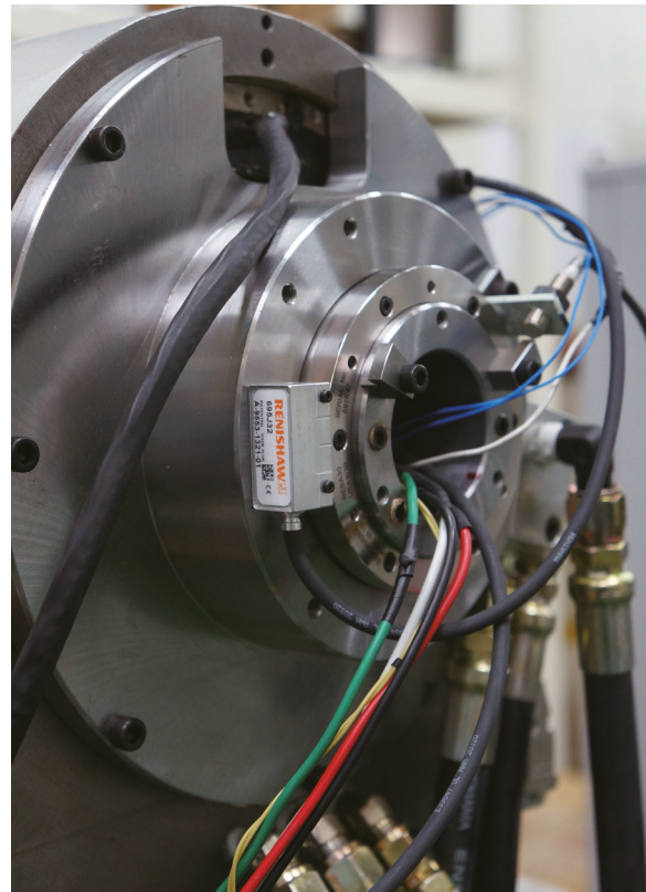
RESOLUTE光學編碼器在傾斜軸上
