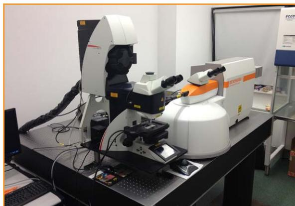
Combined Raman and confocal laser scanning microscope
