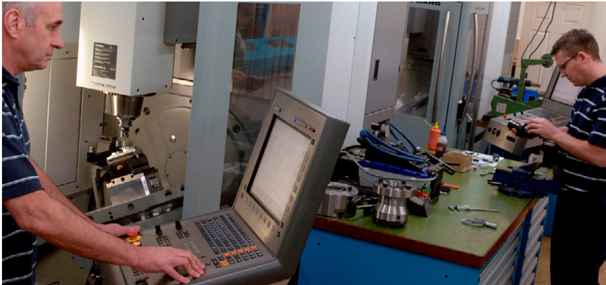
Jobs are loaded onto the DMG DMU-50 machines on small pallets and require multiple tool changes
