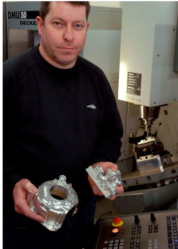
Specialised parts produced on DMG DMU-50 VMCs
